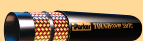
Parker 351TC Hose TOUGH COVER Parker 351ST Hose SUPER TOUGH SAE 100R17. ISO 11237-1 Type R17 Bonded Hose. 3000 PSI Constant Working Pressure. Abrasion-Resistant "Tough Cover" or "Super Tough" cover. 43 Series fittings.
