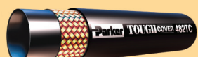
Parker 482TC Hose TOUGH COVER Parker 482ST Hose SUPER TOUGH SAE 100R1 Type AT. ISO 1436-1 Type 1SN. EN 853 Type 1SN. Abrasion-Resistant "Tough Cover" or "Super Tough" cover. 43 Series fittings and Field-Attachable 42 Series fittings.
