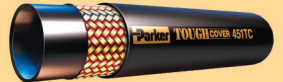
Parker 451TC Hose TOUGH COVER Parker 451ST Hose SUPER TOUGH SAE 100R17. ISO 11237-1 Type R17. 3000 PSI Constant Working Pressure. Abrasion-Resistant "Tough Cover" or "Super Tough" cover. 43 Series fittings.
